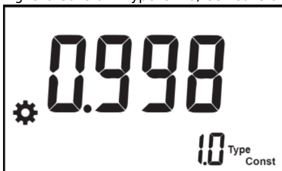
Fig. 5-7 Constant Type is 1.0, Cell constant is 0.998
