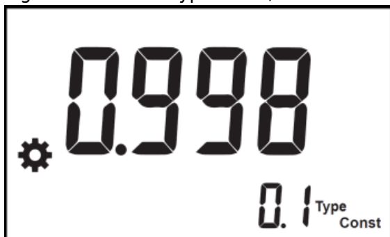
Fig. 5-8 Constant Type is 0.1, Cell constant is 0.0998
