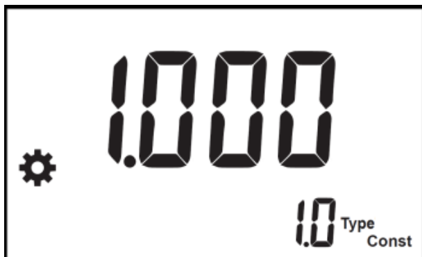
Fig. 5-6 Constant Type is 1.0, Cell constant is 1.000
