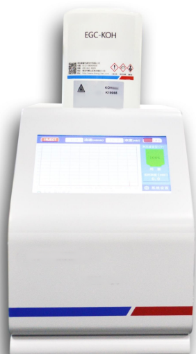
Figure 2-4 External view of eluent generator
