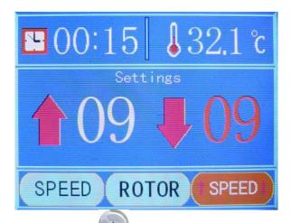
② Press the " UP" button to adjust the acceleration of the rotating speed, or touch the screen and click the icon to do the same operation. There are 10 acceleration levels: 0 is the slowest while 9 is the fastest.
