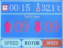
①Press the DOWN" button to adjust the deceleration of the rotating speed, or touch the screen and click the icon to do the same operation. There are 10 deceleration levels: 0 is the slowest while 9 is the fastest. As it is shown below:
