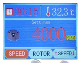
①Press the " UP" or " DOWN" button to adjust the rotating speed value.
