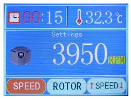
3) On the bottom of the first adjustment panel, press the "SET" SET" button to enter the second adjustment panel (the adjustment panel of rotor modes), or touch the screen and click the rotor number area to enter the same panel. As it is shown below:
