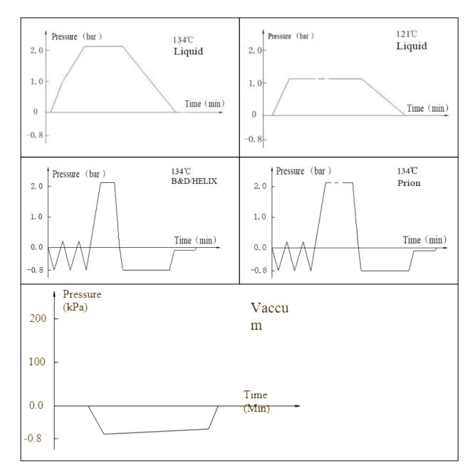
Program operation flow: Start -- pulsating vacuum -- heating -- sterilization -- exhaust -- pulsating vacuum drying -- end
