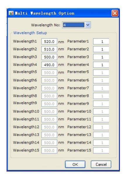
3. Input wavelength number, and Input coefficient: Results = Abs(wavelength 1) × factor 1 +Abs(wavelength 2)×factor 2 +Abs(wavelength 3)×factor 3 +..... 4. Click <OK> button to complete configuration. 5. Put reference sample into light path, select the main menu <operation> <set zero /full-scale> or
