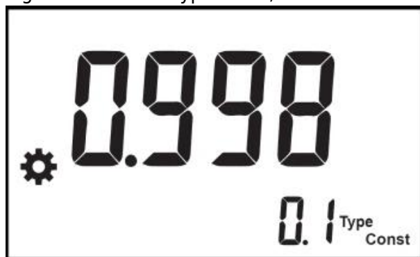
Fig. 5-8 Constant Type is 0.1, Cell constant is 0.0998
