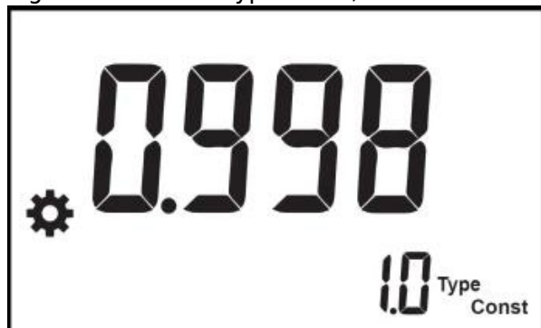
Fig. 5-7 Constant Type is 1.0, Cell constant is 0.998
