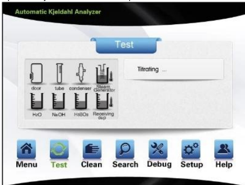
Figure 20 In case discharging and cleaning are set in [Setup], then system will automatically discharge and clean after completion of titration. The cleaning of digestion tube and receiving cup will be respectively carried out following the discharging of the same. The system can not suspend or back upon commencement of cleaning or discharging till the completion of cleaning or discharging.
