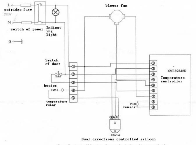
The electric illustrative and wiring diagram of the electronic heating incubator box
