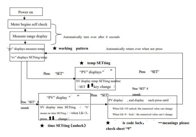
The modification of the temperature controlling parameters
