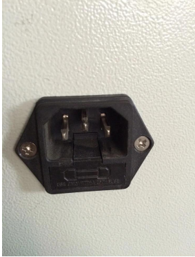
Figure 6 (Total power supply+ fuse)
