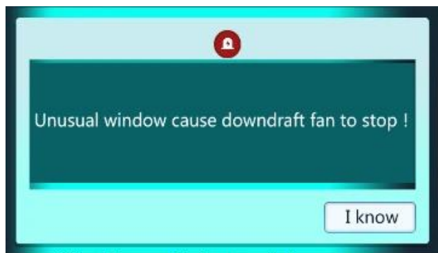
(5) Abnormal front window causes the blower to stop running
