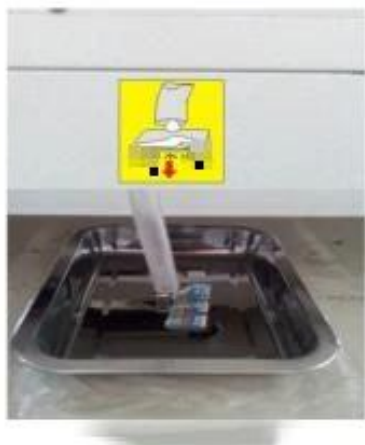
Figure 8 machine condensate water exit
