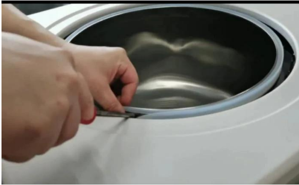
Figure 12 Step 1: take out the sealing ring (Use a slotted screwdriver)
