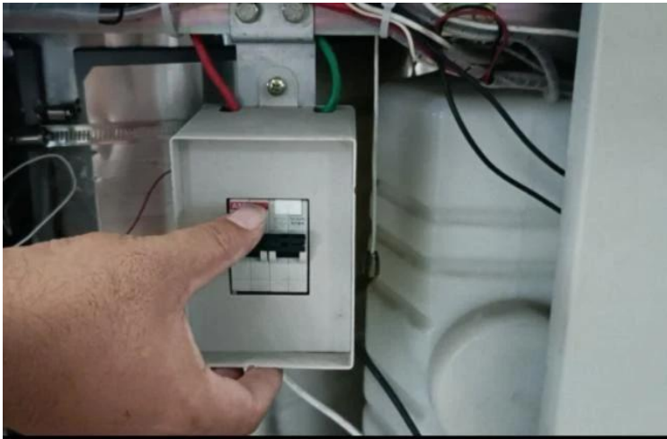
Figure 9 step 4: disconnect the instrument circuit breaker
