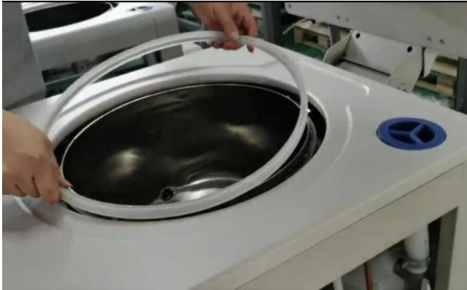
Figure 13 step 2: put on a new sealing
