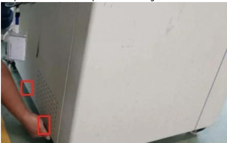
Figure 11 step 6: unscrew the lower screws and open the left and right side plates
