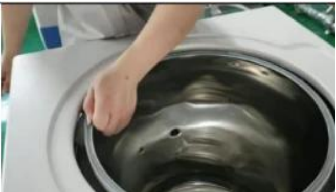
Figure 15 step 4: check whether the whole seal ring is flush with the chamber edge
