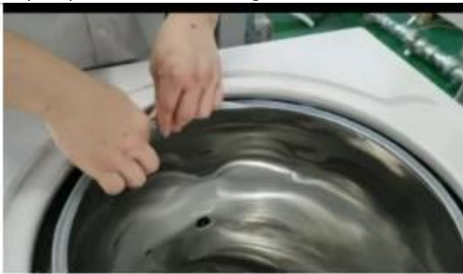
Figure 14 Step 3: press the seal ring edge flush
