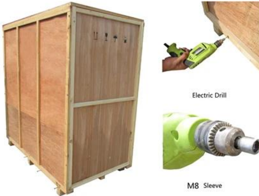
Figure 1 Method 2 Use M8 wrench to unpack
