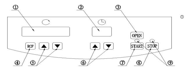
Speed/RCF/Rotor No. screen ② Timer screen ③ open the lid ④RCF ⑤+/- key for speed ⑥+/- key for run time ⑦Start the centrifuge ⑧ Stop the centrifuge ⑨ start light and stop light
