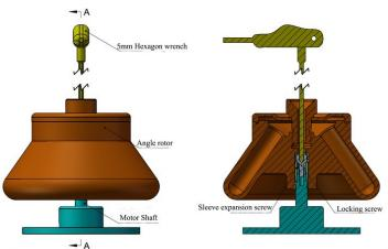
Do remember,we can tighten the rotor only after the rotor is installed fully down to the shaft.
