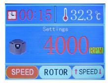
Press the "SET" SET" button to enter the rotating speed adjustment panel. Next, press the " UP" or " DOWN" button and press the " SET" SET" button again to enter the time adjustment area. The needed minutes can be chosen by pressing the " UP" or " DOWN" button.
