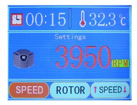
Press the "SET" button to enter next step, and the needed hours can be chosen by pressing the "DOWN" button.
