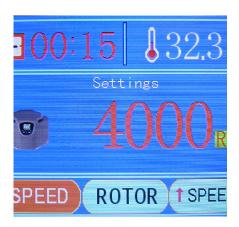
a) Press the " Tup" or " DOWN" button to adjust the rotating speed value.
