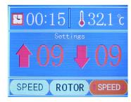
a) Press the " DOWN" button to adjust the deceleration of the rotating speed, or touch the screen and click the icon to do the same operation. There are 10 deceleration levels: 0 is the slowest while 9 is the fastest.
