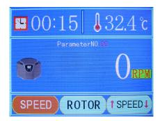
2. Press the SET "SET" button to enter the first adjustment panel, or touch the screen and click the rotating speed area to enter the same panel.
