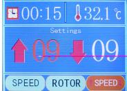
b) Press the " <a> UP</a>" button to adjust the acceleration of the rotating speed, or touch the screen and click the icon to do the same operation. There are 10 acceleration levels: 0 is the slowest while 9 is the fastest.
