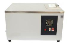
The instrument is newly designed and is suitable to determine solidifying point of petroleum products. It is widely used in oil exploitation companies, petroleum manufacturers, petroleum users, colleges and scientific research institutes. The material of workbench is stainless steel. It adopts special technology. It is no need to use cooling liquid in cold chamber. The cooling rate is fast and efficiency is high. The instrument adopts bench structure. The design is simple and easy to use.
