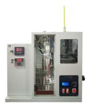
The instrument is suitable to determine the distillation characteristics of wax oil, lubricating oils and other petroleum products with high boiling point range. It adopts single chip microcomputer technology, can automatically control the vacuum pressure.
