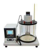
The instrument is suitable to determine kinematic viscosity of liquid petroleum products (Newtonian fluids )at a constant temperature. This instrument adopts hard glass bath and electric stirring device. Easy to observe the sample. The temperature in water bath is uniform.
