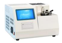
The instrument is specially suitable to determine different kinds of colored paints, oil paints, adhesives, solvents and petroleum products which the closed cup flash point is -30°C~50°C. It can realize purpose of testing closed cup flash point rapidly and at low temperature. Test sample needed is less 2ml for each time(4ml for solid sample and semi-solid sample). The determination procedure is automatically completed except ignition. Test results can be printed automatically.
