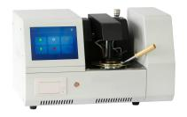
It adopts an 8-inch IPS high-definition capacitive screen. Temperature rise, cover opening, ignition, detection and printing data are completed automatically, and the test arm rises and falls automatically. Electronic ignition, gas flame, automatic air cooling at the end of the test.
