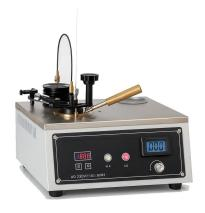
The heating power is continuously adjustable. The power is shown visually by voltmeter. The temperature control mode is advanced and reasonable. The structure is designed small and exquisite. The stainless-steel table board is beautiful and easy to clean. Operation is easy. Test results are precise. It has been chosen as the instrument to test the closed cup flash point by many metering and detecting institutes.
