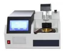
The instrument adopts LCD screen to display. It is applicable to all petroleum products with flash points above 79°C and below 400°C except fuel oils. Differential coefficient detection. Automatically correct the system deviation.
