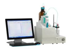
The instrument can accurately detect the acid value of transformer oil, turbine oil, anti oil, diesel, gasoline and other petroleum products. Test results can be saved as word and excel format documents. It adopts the original imported titration device, and the detection signal is stable and reliable. The instrument can clean, replenish and add liquid automatically.
