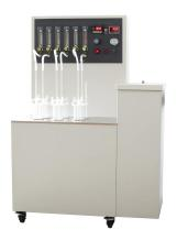
The instrument is suitable to determine the oxidation stability of distillate fuel oils with accelerated method. It adopts metal bath structure. No need to add water during determination. Clean and eco-friendly. Easy to operate. It is the preferred automated instrument to determine the oxidation stability of distillate fuel oils for the units of petroleum mining, producing and using and other relevant colleges and scientific research institutions.
