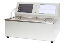
The instrument is used to make determination for vapor pressure of gasoline, volatile crude oil and other volatile petroleum products. It cannot be used to determine the vapor pressure of LGP. It is fully-automatic vapor pressure tester by PC control and operation. Advanced heating technology do separation of water and electricity meanwhile lower the height of water in bath. No blind angle in bath. It can save water and energy and also convenient to be cleaned.
