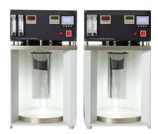
The instrument is used to determine the foaming tendency and stability of lubricating oils. he instrument adopts all-in-one structure. It includes three parts: low temperature test part and it's control, high temperature test part and it's control, a portable cooler for low temperature test part. The instrument equips an automatic timing alarm.
