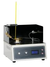
It adopts special heating furnace to ensure the safety of test. It is applicable to all petroleum products with flash points above 79°C and below 400°C except fuel oils. The heating power is continuously adjustable. It can meet requirements of test. The instrument is fully self-contained complete. The operator can do determination as long as connecting with coal gas or other civil gas. With fast cooling function, it can improve test efficiency.
