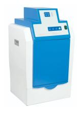
The zoom, focus, aperture, UV light and white light can be controlled by PC. Auto-delay-shutdown function for UV light.
