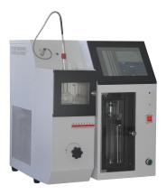
Big LCD screen, which can show distillation rate, temperature, recovery volume ratio etc.
