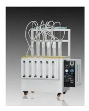
The glass test tube meets the requirements of ASTM standards; Electronic timer, digital display, with alarming; Precision flow meter regulates gas flow, separate flow control; Six test tubes can work at the same time, with fan cooling; Three-dimensional Structure; Stainless steel heater, heating bath; Imported Omron PID temperature controller, digital display temperature, accuracy 0.1 °C
