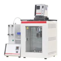
The instrument is a split type, including a heating bath and an accurate flow meter; High temperature resistant borosilicate glass cylinder,  $\Phi$ 300 x 450mm, meets the requirements of the standard;
