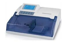
User friendly operation system with large LCD display. Washes flat, U and V-bottom strips and plate. 12-way or 8-way manifold, automatic and manual positioning. Large memory, up to 100 wash protocols can be programmed. Multi-channel, 1 or up to 3 for wash, 1 for rinse and 1 for waste. Plate shaking function, time and speed are adjustable. Two 96-well plate incubation positions (optional). Liquid level detection and alert function. Easy maintenance.
