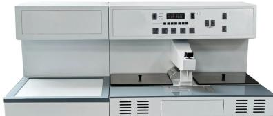
The Embedding center is composed of two modules, main console and Cryo Console. It is independent design, can put the position left-to-right or right-to-left, to meet different habits of customers. The large working surface allows user processing many samples at the same time. The temperature and work start time can be settable through the control panel.
