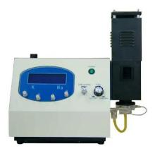
It meets the requirements of medical clinical test in addition to new added functions of testing high connected K and Na it has the detection function of Li salt taken by the mental patients.
