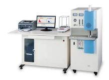
It can accurately measure the carbon and sulfur in steel, iron, alloy, nonferrous metals, and other materials.
