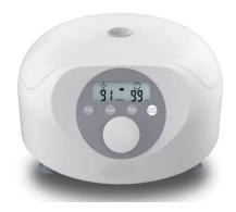
Pulse operation for fast and convenient quick spins; Speed up to 15000 rpm (15100 x g); Brushless DC motor drive quickly to the target speed; Smooth and quiet operation (noise  $\leq$  65 dB); Automatic door lock and over-speed detection; Wide voltage technology: speed is not affected by voltage fluctuations, high speed accuracy
