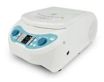
In static pre-cooling mode, when the centrifuge cover is closed, if the set temperature is lower than the ambient temperature, the compressor will automatically starts to cool.
