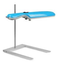
Compact designed, simple operation, one-key switch the wavelength. Lamp wavelength 365nm or 254nm long life. With a battery, it can be used for a long time without electricity. Optional H-type stands fix the UV analyzer to meet special operational needs. H-type stands for optional to fix the instrument, meet the demand of special operations. It can adjust height and angle.
