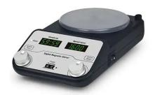
Can stir 50ml-20L standard or non-standard reaction bottles. Equipped with silicone pad upon the working surface, the shell is made of metal, high strength, high temperature resistance, corrosion resistance. Brushless DC motor, stable performance, low noise, long life and no sparks. Exquisite and compact design of the whole machine, 30° bevel control panel is suitable for sitting and standing viewing angles.
