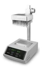
The heater heats the sample rapidly to the evaporation temperature, and at the same time, the gas is blown to the surface of the solution through the gas needle, which promotes rapid evaporation of the solution and concentration of the sample. The height of the air cavity can be adjusted. The length of a standard gas needle is
