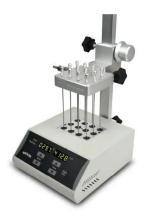
The height of the air chamber plate can be adjusted. The length of a standard gas needle is 150mm.
