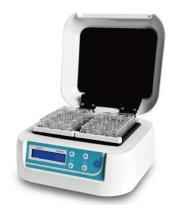
LCD display. Setting temperature and actual temperature simultaneously displayed. Diminishing time displayed.
