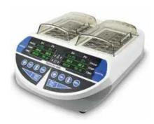
Unique dual temperature control slot can individually control temperature to make sure noninterference. One equipment to meet the demands for more experiments. OLED display, simple interface, double time and temperature setting, simultaneous temperature and diminishing time display.
