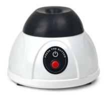
The max. the diameter of the tubes is up to 30mm. Suit for mixing tubes /centrifugal tubes with prominent mixing effect.
