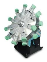
Humanized designed operation keyboard. LED display time and speed. Several optional turntable supplied, suit for the tubes from 1.5ml to 50ml. The turntables' gradient can be adjusted from 0 to  $90^\circ$ . Timing function. Time range from 0 to 9999min, LED display remaining time. Beep alarm when program time ends.
