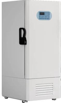
Accurate temperature controller, setting temperature range of -40 to -86°C, and accuracy is 0.1 °C.
