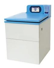
The max capacity of swing rotor is 6x1200 ml.
