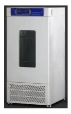
The refrigeration system adopts high-quality well-known brand compressors with time-delay protection function and stable operation. It introduces the concept of green environmental protection and uses fluorine-free R134a refrigerant to make the system more energy-saving and efficient and make the environment healthier; Reasonable air duct circulation system to ensure uniform temperature of working room
