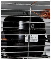
Without fluorine R134a refrigeration compressor
