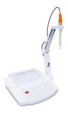
1 to 3 points push-button calibration with auto-buffer recognition Selectable pH buffer group, including the USA and NIST options Automatic electrode slope display helps user decide whether to replace sensor Automatic Temperature Compensation provides accurate reading over the entire range
